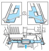
(1) Make sure that the pins on the left and right arms of the embroidery frame holder fit into the positioning slot and hole on the embroidery frame.
